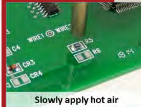
Solder bump and flux both lands
